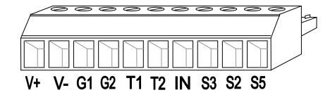
V+ Supply voltage 9-24V DC V-Supply voltage negative polarity (GND) **G1** Simulated line output from the GSM system (to the alarm panel's TIP input) G2 Simulated line output from the GSM system (to the alarm panel's RING input) **T1** Landline (PSTN) input **T2** Landline (PSTN) input IN Direct GSM (to activate, connect to V-) **S3** Reserved **S2** Reserved **S5** Reserved
