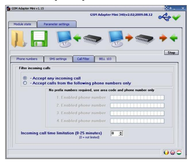
The GSM Adapter Mini is able to manage calls coming in through the GSM network, and to ring up devices (telephone, alarm system) connected to it. With this, it can receive incoming GSM calls in places where there is no PSTN line extension by means of a simple analogue telephone.
