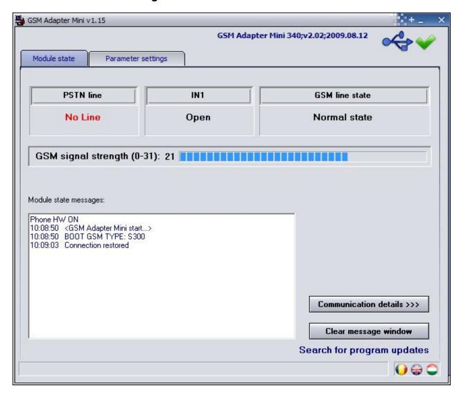
When connected, the module's current state can be monitored in the "Module state" window. The following information are displayed: the availability of landline phone, state of the input, the GSM line state, the GSM signal strength and the module state messages. The module message window can be cleared by pressing "Clear message window" button.
